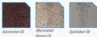
Photo shows NMMA FC-W Corrosion Test performance on Mercury cylinder strips.
